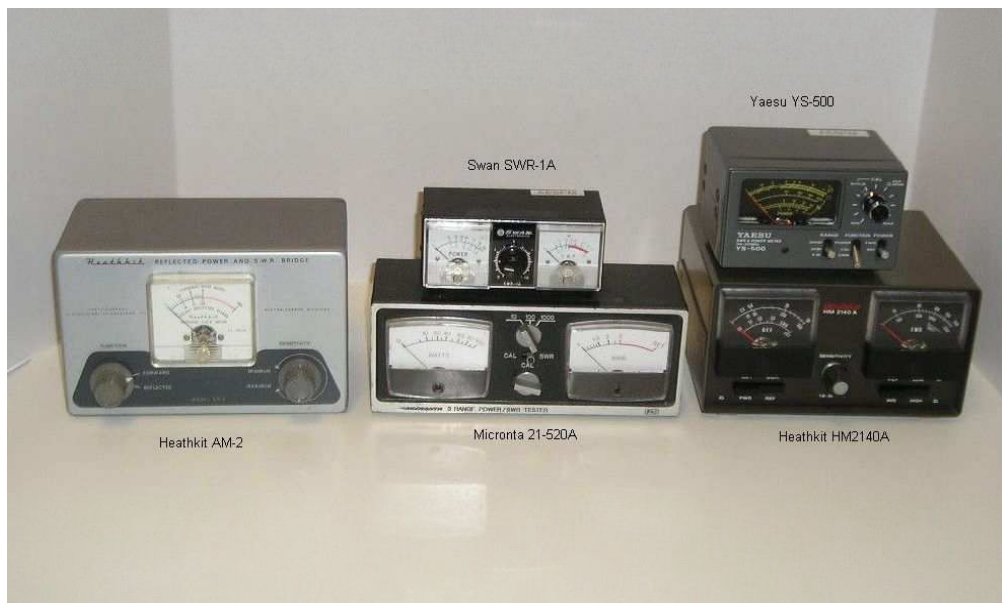
Fig.1. Typical SWR Meters Found at Swap Meets. Clockwise from left, the Heathkit AM-2, Swan SWR-1A Yaesu YS-500, Heathkit HM2140A and the Micronta 21-520A.
