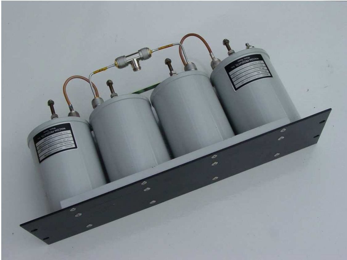
Fig.1. A 4-resonator duplexer similar to the one used on the W6UU 70-cm repeater. A unit like this costs about $1,800, has an insertion loss of 1.0 dB or less and isolation of 90 dB. A set for 2-meters is much larger than this. A resonator for 6-meters approaches the size of a trash can. The panel in this photo is 19" wide.
