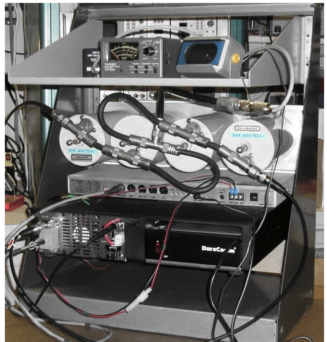
Fig 2. Rear view of the test rack. The speaker, SWR meter and dummy load on the rack shelf are not part of the repeater.
