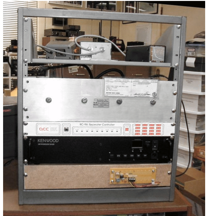
Fig. 1. Repeater components mounted in the test rack. From the bottom up, s-meter signal conditioner, Kenwood repeater, RC-96 controller and the duplexer.
