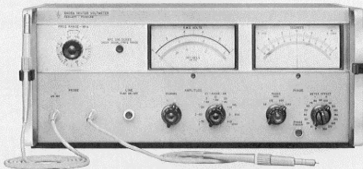
Fig. 1. —hp— Model 8405A Vector Voltmeter measures amplitudes and phase simultaneously. Instrument has frequency range of 1 MHz to 1 GHz, sensitivity of 100 \mu V full-scale, dynamic range of 95 dB, phase resolution of 0.1°, and is simple to operate. Thus it makes feasible many measurements which formerly were difficult or impossible.
