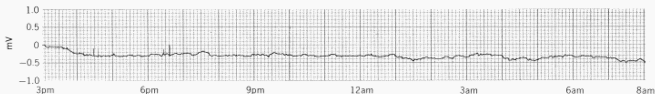
Fig. 5. Typical zero stability of -hp- Model 427A Voltmeter. Record was made in laboratory environment subject to usual temperature fluctuations of \pm 2^\circ\text{C} .
